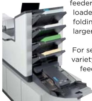
For secure feeding of a wide variety of printed paper, the feeders use mechanical doubles detection.
